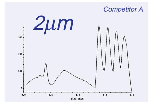
A six component library analyzed with an extremely fast gradient on a HAISIL HL C18 5µm 50x4.6mm column (top) and Competitor A's new 30x4.6mm 2µm column (bottom).
